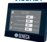
7" HMI color widescreen panel touchscreen with Ethernet interface
